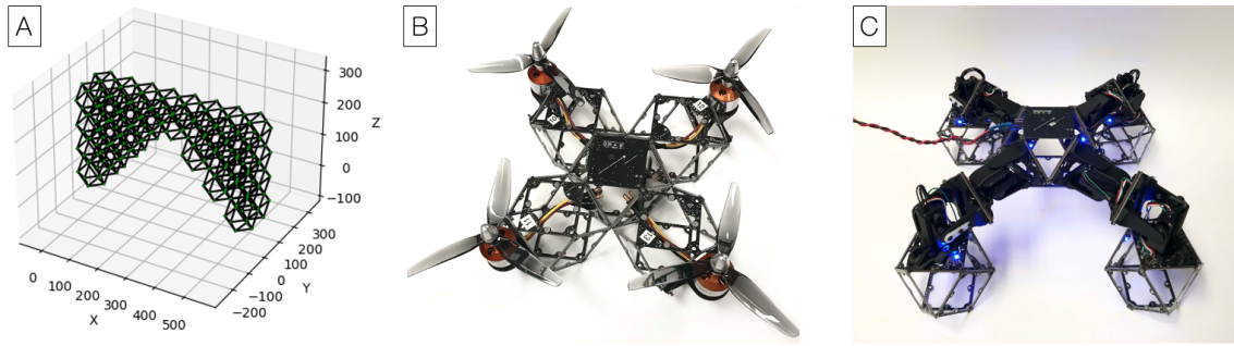
Figure 4-1: Immediate next steps. A) Plot of a small voxel bridge. B) Partially assembled voxelcopter. C) Partially assembled ant robot.
