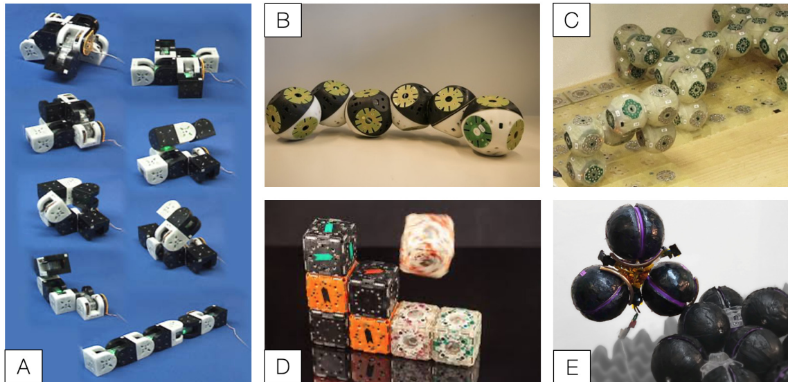
Figure 1-4: Example modular robotic systems. A) M-TRAN III [22], image from [26]. B) Roombots [23], image from [27]. C) Soldercubes, image from [28]. D) M-Blocks [24], image from [29]. E) FireAnt3D, image from [25].
