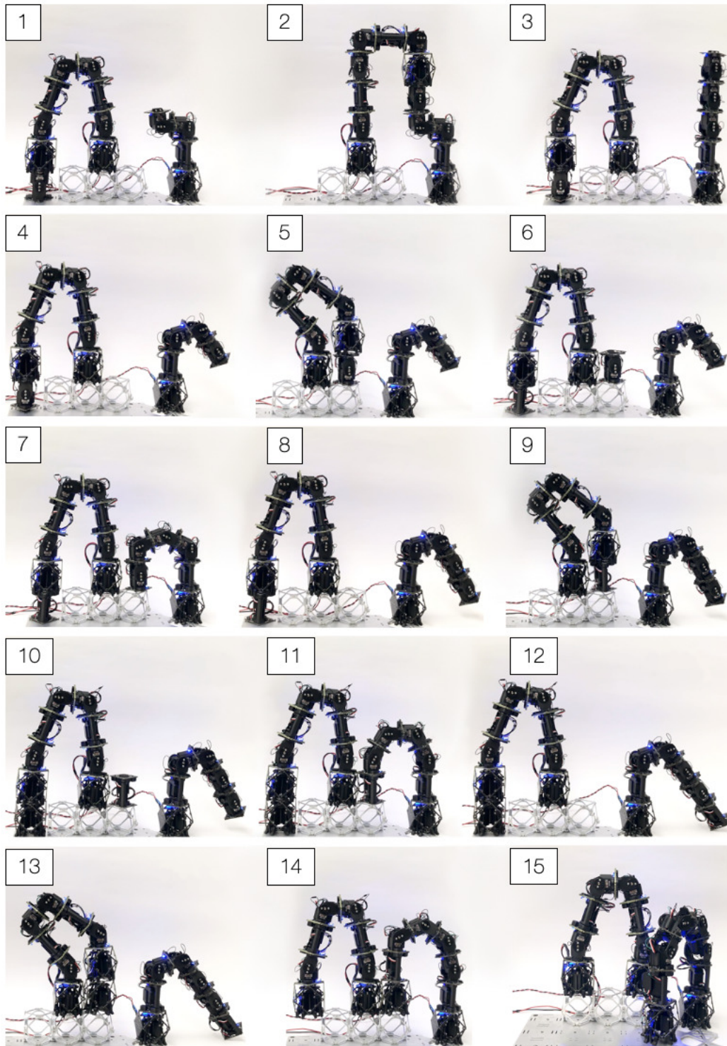
Figure 2-23: Second half of freeze frames from the robotic assembly of a second robot.
