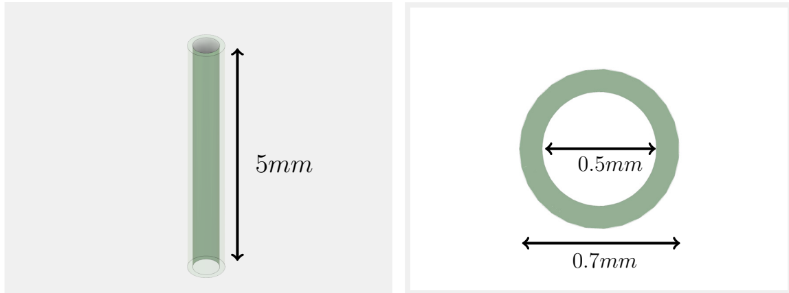
Figure 4-21: Schematic diagram showing the dimensions of the MAS diamond rotor probe.
