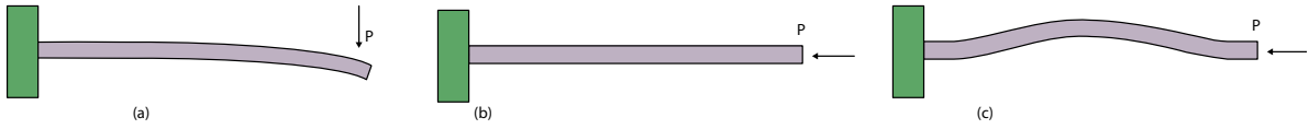
Figure 3-5: (a) Applied bending load; (b) applied axial load; (c) axial load sufficient to induce buckling.
