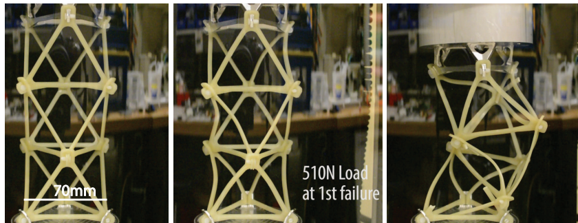
Figure 6-10: Mechanical testing of octa-stack under position controlled loading. The middle image just before failure due to buckling. The right-most image is near total failure, half of the struts have already broken.
