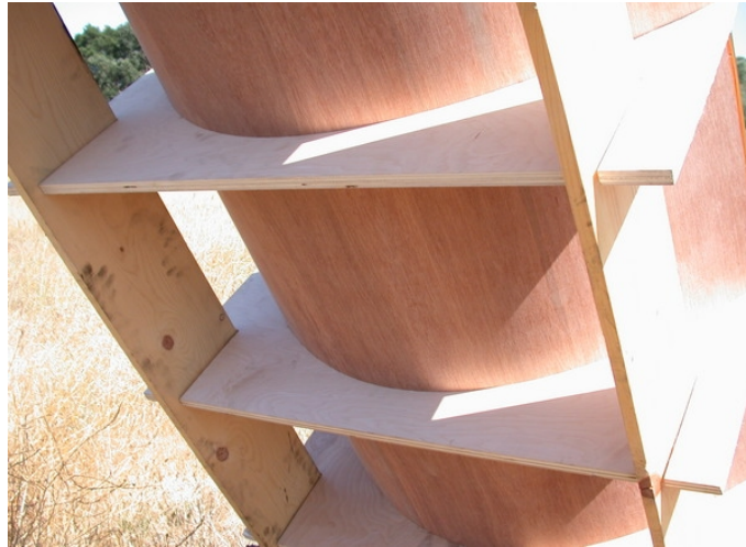
Figure 10: Stiffening the reflective surface of the trough using thin plywood screwed into the shaping ribs. (Seven Troughs, Nevada)
