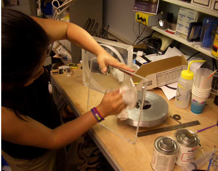
Figure 20: Cleaning the acrylic end plate prior to bonding
