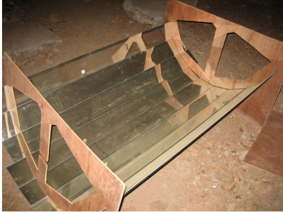
Figure 8: One night's dirt accumulation on trough. (Pabal, India)
