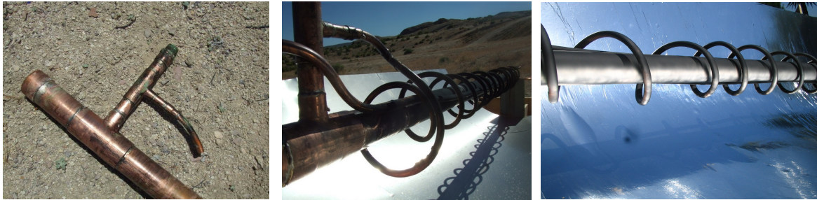
Figure 11: Steam generator made from 2.5" diameter copper pipe. Left showing fill and steam exit "T" in boiler. Center and right showing steam reheat coils.
