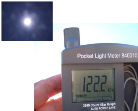
Figure 1: Measuring solar irradiance with a light meter.
