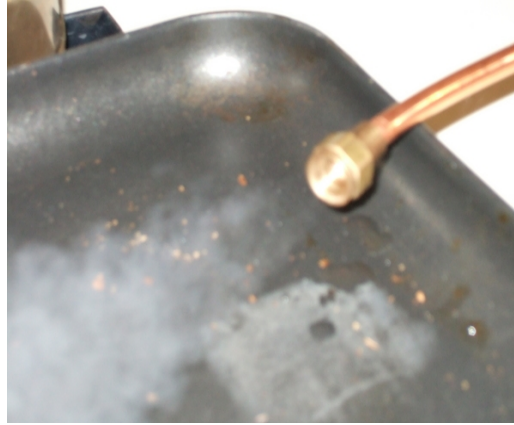
Figure 13: A well formed jet of steam from the pressure cooker boiler.
