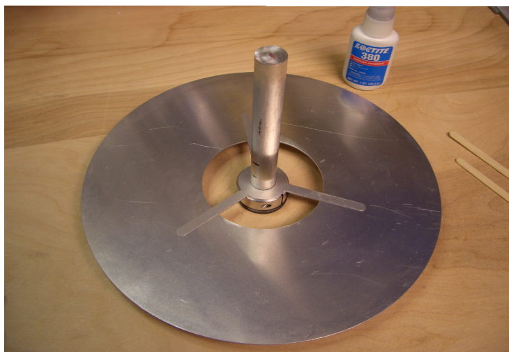
Figure 19: Assembling the disc pack onto the shaft
