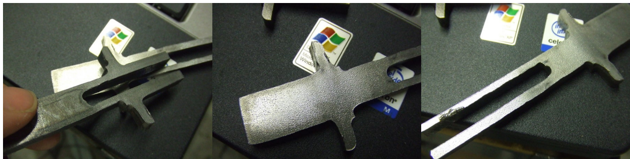
Figure 27: Plasma cut medium steel shaft. Plasma cutting was unable to give straight perpendicular cuts necessary for this design.
