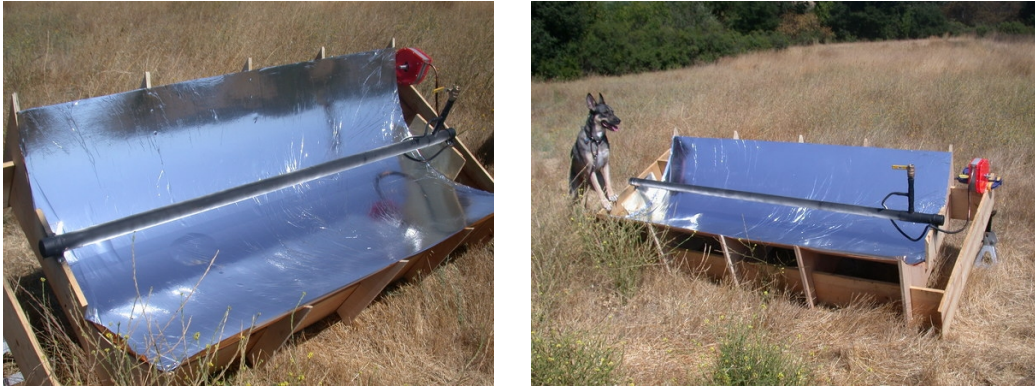
Figure 3: Integrated solar collector, boiler, and turbine. (Calero State Park, California)
