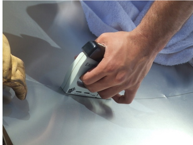
Figure 7: Stapling aluminum flashing to shaping ribs to form parabolic reflector trough.
