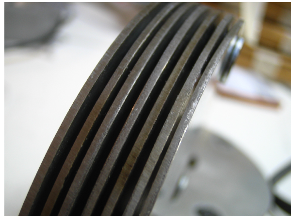
Figure 24: Deformation of a stainless steel disk, probably occurred during machining.
