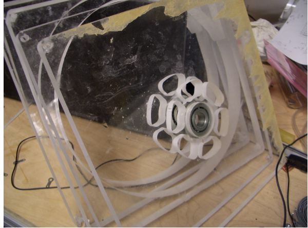
Figure 16: Acrylic housing and end plates with pressed-in steel bearings.
