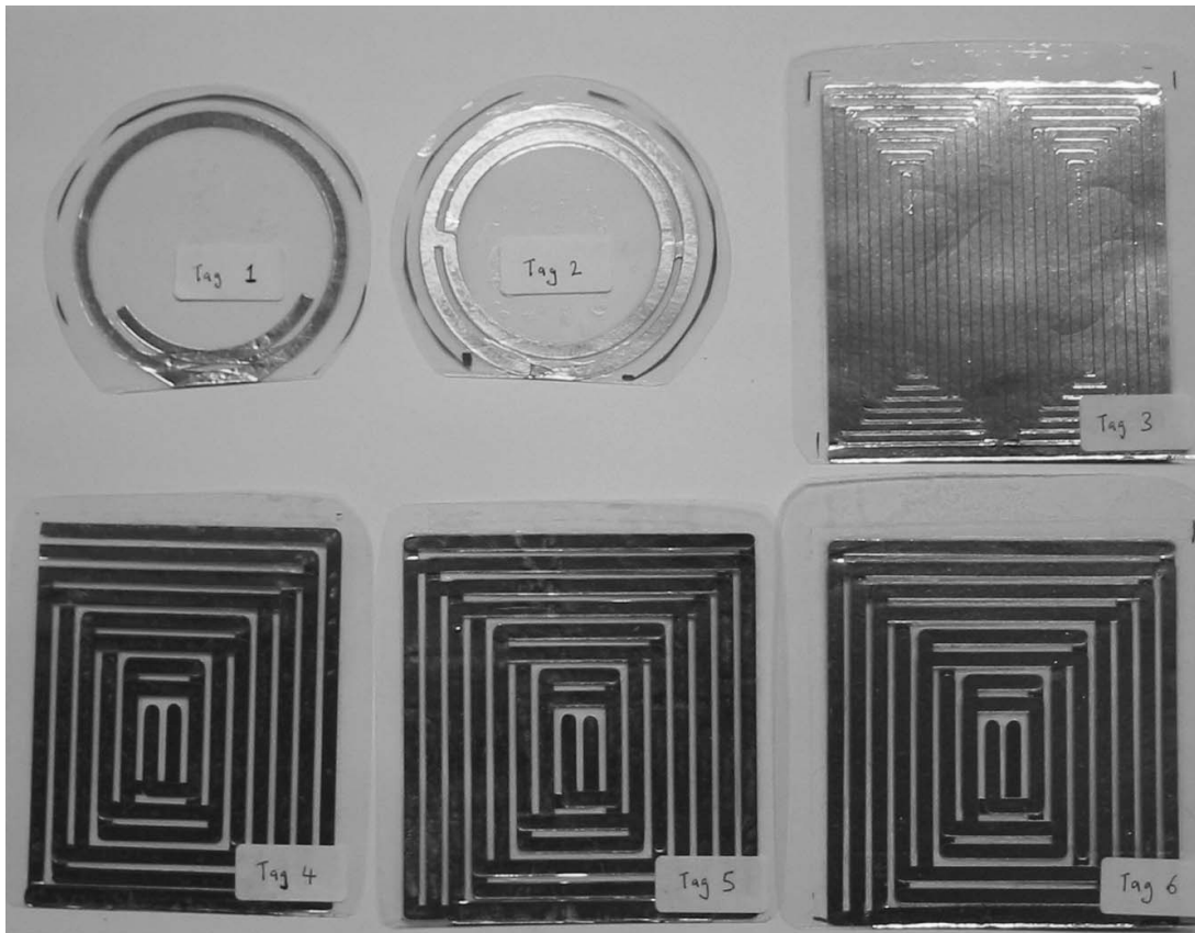
Figure 24. The 6 Chipless Materials-based Tags Used to Evaluate the Network Analyzer Board
