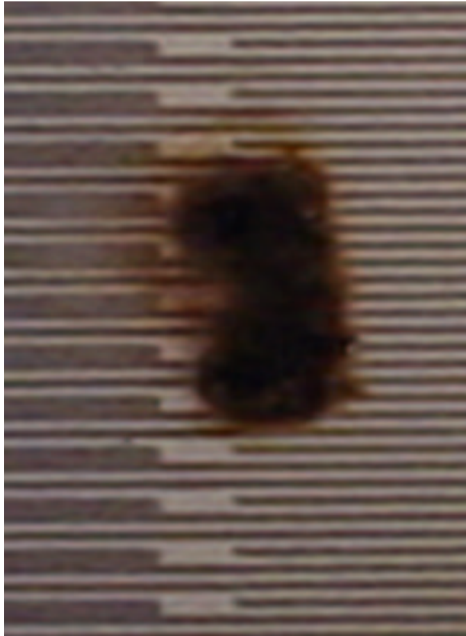
Figure 3-9: The result of dielectric breakdown between electrodes
