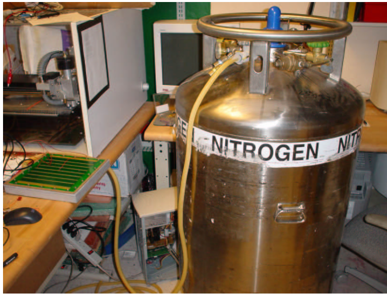
Figure 4-11: Liquid nitrogen cylinder used to test air bearing.
