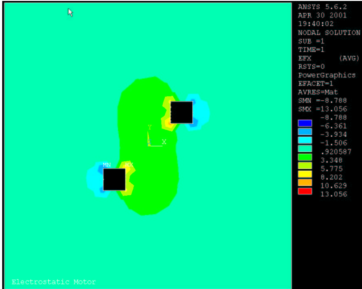
Figure 4-1: ANSYS model of electric field in the x-direction between two electrodes
