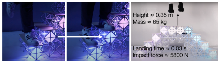
Figure 17: The stair lights' step-response behavior and the approximate jump impact force calculation.
