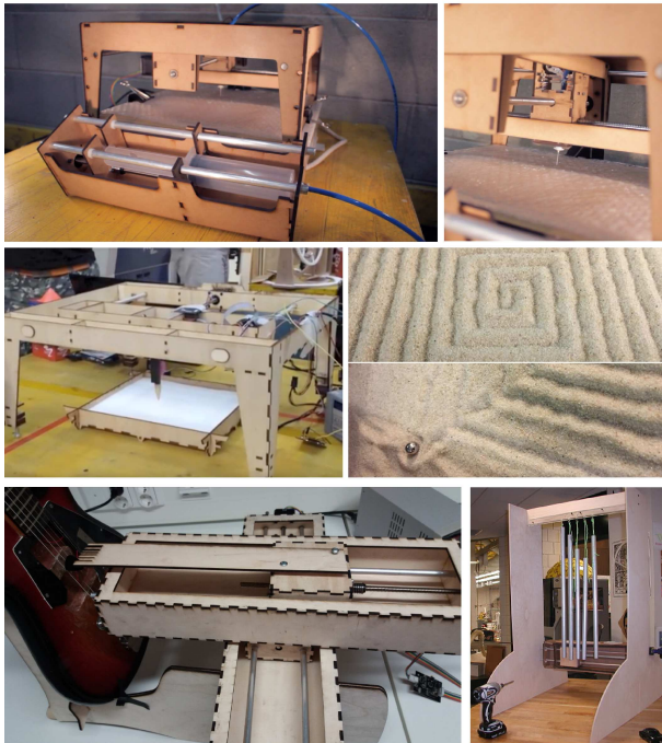
Figure 14. Odd machines produced included a machine that injects coloured liquid into bubble wrap bubbles to make a kind of dot-matrix printer by Fablab Torino (top); sand gardening machines by Opendot Milan and the LCCC Fablab (middle); and music making machines by the Oulu and LCCC Fablabs (bottom).
