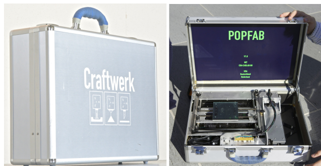
Figure 6. Popfab's z-axis folds down to fit into a briefcase.
