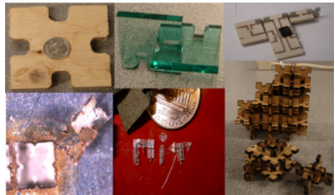
Figure 3 GIK parts made out of different material: plywood, Plexiglas, aluminum and fiberglass composite material, stainless steel, transparency (celluloid) and cardboard.
