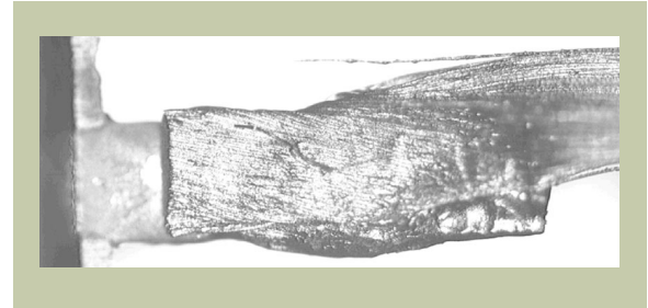
Figure 16 Top view of a stainless steel thread welded to Cu/CuSnPb lead
