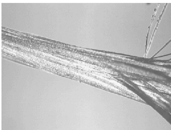
Figure 11 Photomicrograph of Bekintex single-ply continuous-drawn stainless steel fiber bundle
