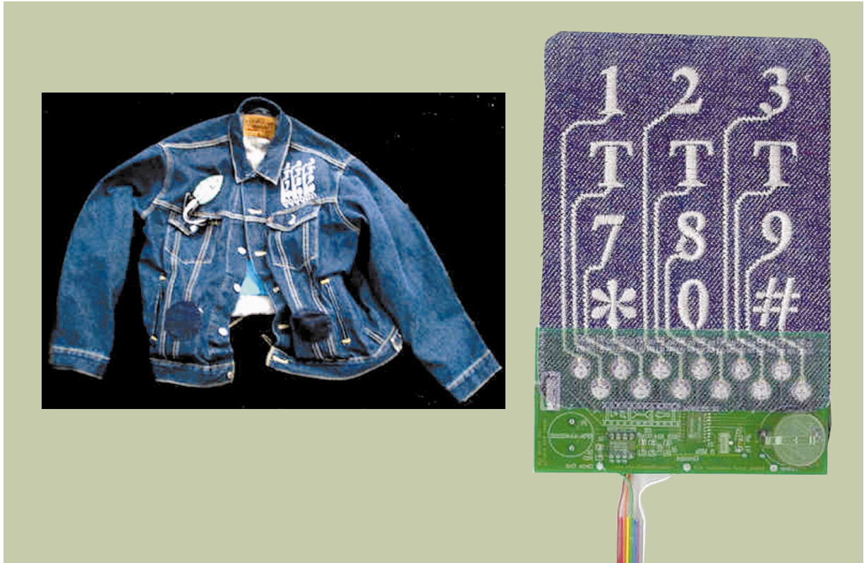
Figure 3 On the left is the Musical Jacket, comprising a fabric keypad on one side, a MIDI synthesizer “boat” on the other side, speakers behind speaker grills in the pockets, and fabric buses visible inside the jacket. On the right is a composite image of both sides of the circuit board attached to the back of the fabric keypad.
